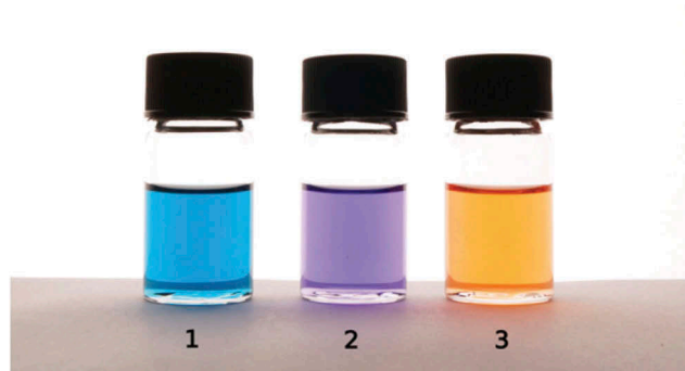
Figure 2. (Colour online) Photograph of solutions of the dyes at ca. 1 \times 10^{-4} \text{ mol dm}^{-3} in dichloromethane.
