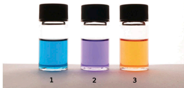
Figure 2. (Colour online) Photograph of solutions of the dyes at ca. 1 \times 10^{-4} \text{ mol dm}^{-3} in dichloromethane.
