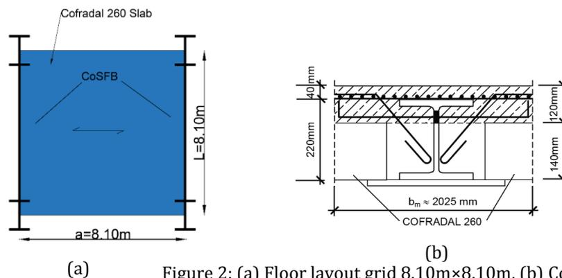
Figure 2: (a) Floor layout grid 8.10m×8.10m, (b) CoSFB with Cofradal 260mm flooring system section (Braun et al., 2011)
