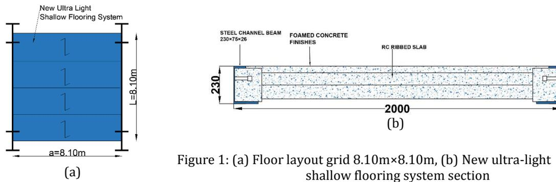
Figure 1: (a) Floor layout grid 8.10m×8.10m, (b) New ultra-light shallow flooring system section
