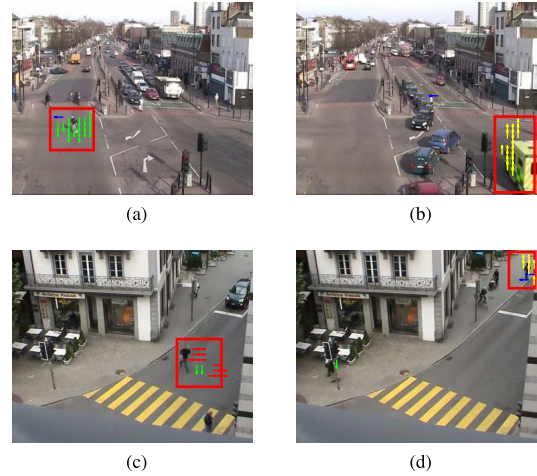
Fig. 11. Example of anomalies localization. The red rectangle is the manual localization. The arrows represent the visual words with the smallest marginal likelihood, the locations of the arrows are the results of the algorithmic anomaly localization. (a) and (b) Examples of anomaly localization for the QMUL data. (c) and (d) Samples of anomaly localization for the Idiap data.
