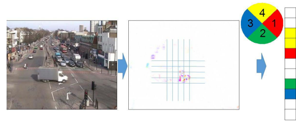
Fig. 1. Structure of the visual feature extraction. From an input frame (left), a map of local motions is calculated (center). The motion is quantized into four directions to get the feature representation (right).
