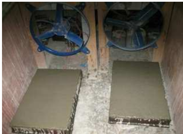
(b) Test set-up for plastic cracking measurement
