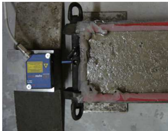
(b) Test set-up for shrinkage measurement
