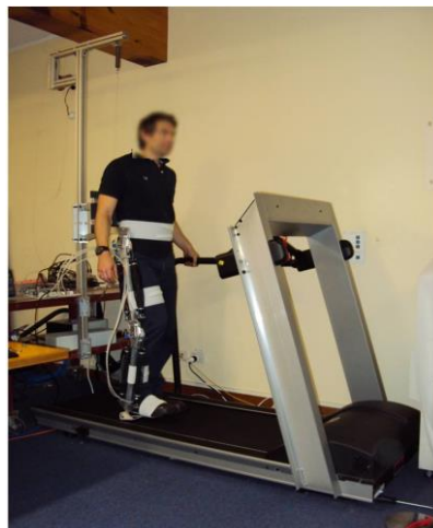
Fig. 1. Experimental setup of the robotic orthosis with a subject walking on a treadmill.
