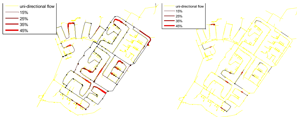
20 Figure 4. Fraction of time that flow reverses in a model with (left) bottom-up allocated with SIMDEUM demands (Blokker 2010); and (right) top-down demand allocations. 50% means 50% of the time flow is in one direction and 50% in the other.
