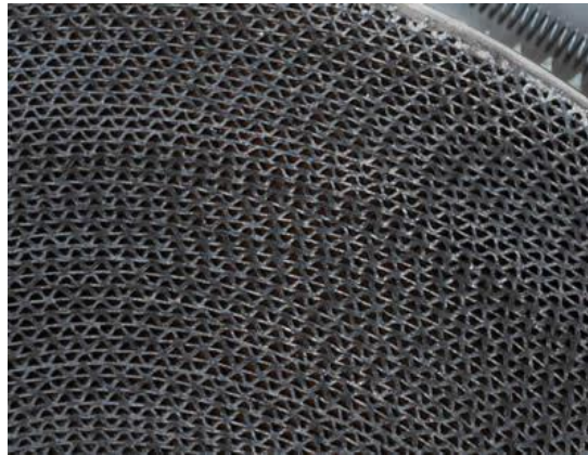
Figure 1 –Section of the matrix of a desiccant wheel for mechanical HVAC
