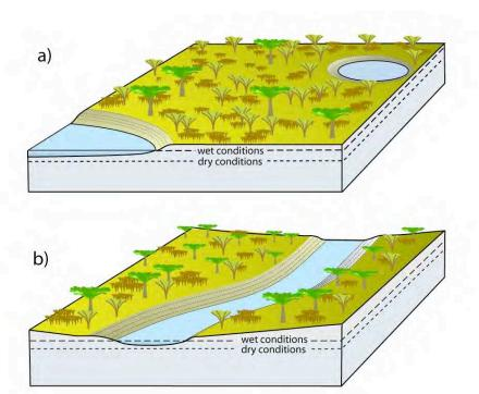
Figure 1 Schematic illustration of effects of changing water table in flat landscapes
