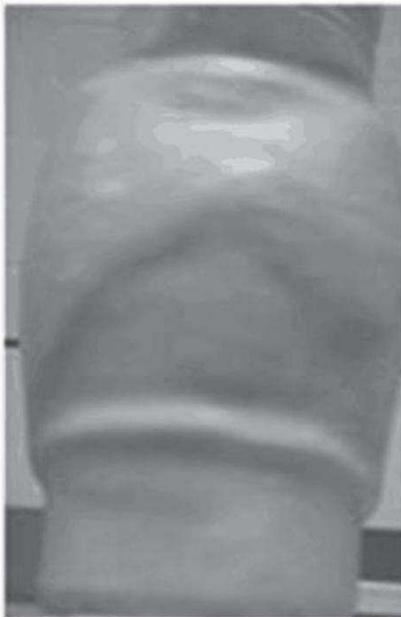
Figure 12. Images of numerical (top) and laboratory (bottom; Marri et al., 2012) cemented specimens after shearing to 20% axial strain under 1MPa (a) and 12MPa (b)
