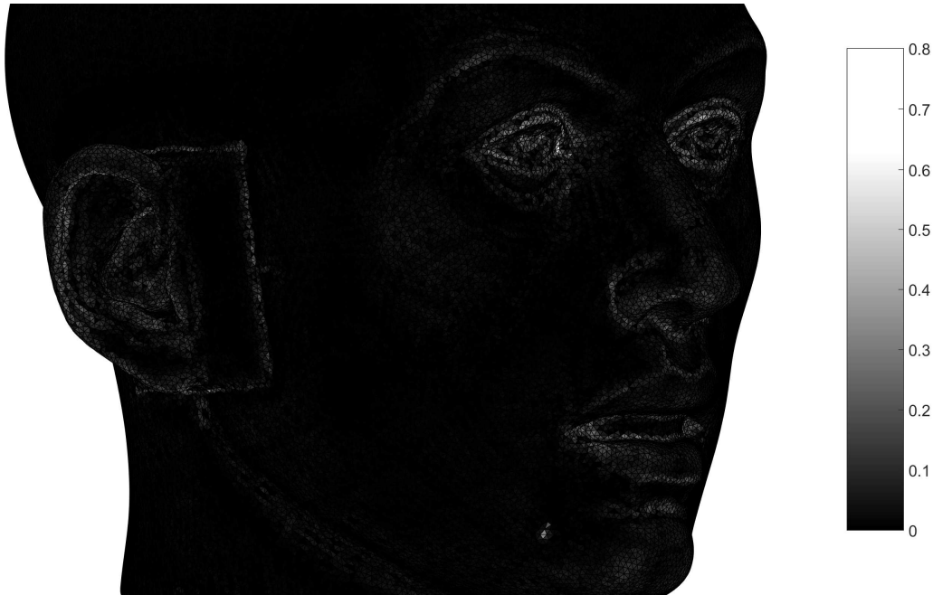
Figure 8: Distances in mm between the two meshes, plotted on the final mesh as a colourmap
