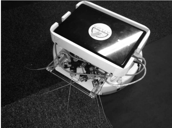
Figure 2: CrunchBot, a whiskered mobile robot platform.
