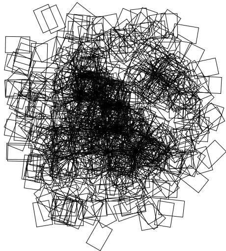
Figure 13: Montage showing the collection of inferred tables from each independent robot pose, for very noisy ( \sigma_r = 0.5, \sigma_\theta = \pi/8 ) sensors.
