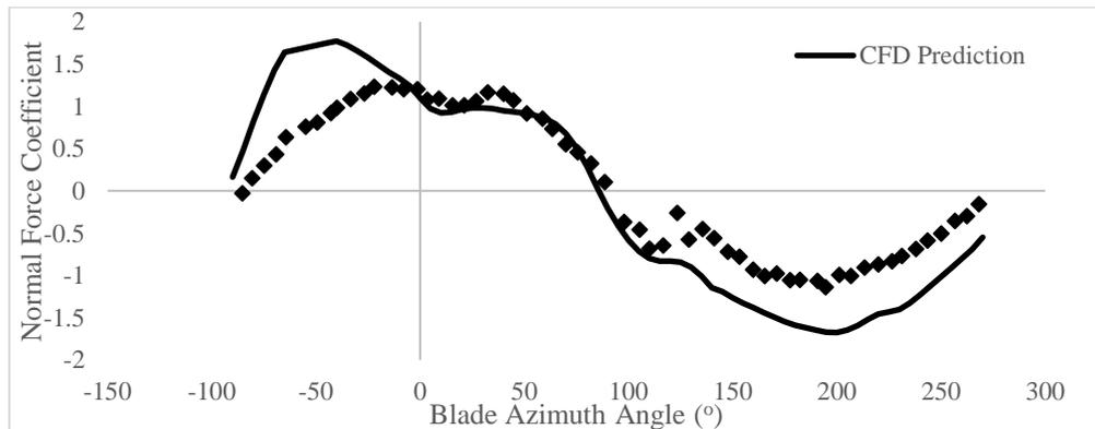
Figure 1: Comparison for CFD predictions against experimental data of the Normal Force for the High Speed case
