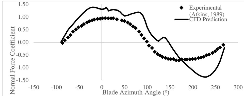
Figure 2: Comparison for CFD predictions against experimental data of the Normal Force for the Low Speed case
