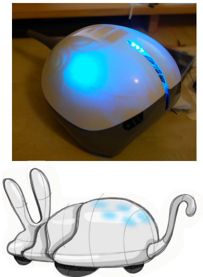
Figure 3. (Top) MIRO is equipped with six LEDs under its body shell through which it can display arbitrary light patterns in a bid to communicate affect. Here shown in blue, neutral mode. (Bottom) Prototype artwork showing original conception of signaling LEDs.
