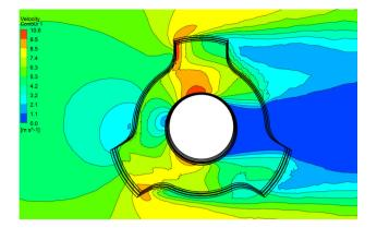
Fig. 7 Plan view of air velocity at a height of 250 m
