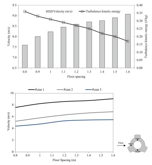
Fig. 11 Effect of floor spacing on wind speed at different points
