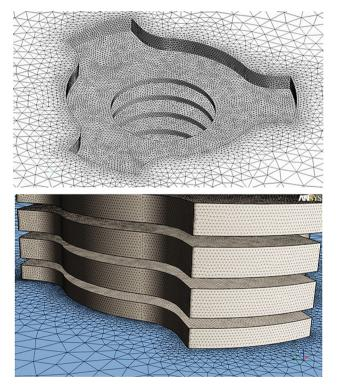
Fig. 3 Mesh generation on the computational domain
