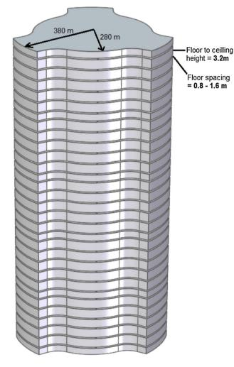
Fig. 1 Section-front view (1.6 m distance between each floor)
