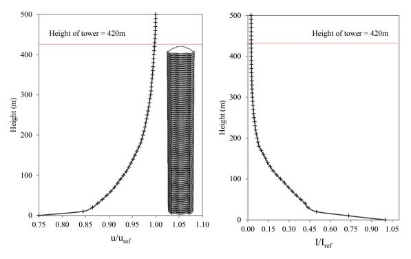
Fig. 5 Representation of the boundary layer profile and turbulence intensity
