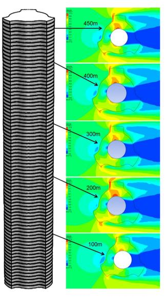
Fig. 9 Velocity distribution on the building structure at increasing altitude
