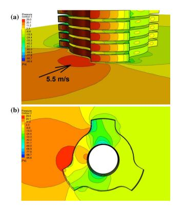
Fig. 6 Contour levels of static pressure at a height of 250 m on the **a** building fabric **b** plan view
