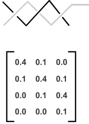
Fig. 7: The GLI Matrix of two linkages.
