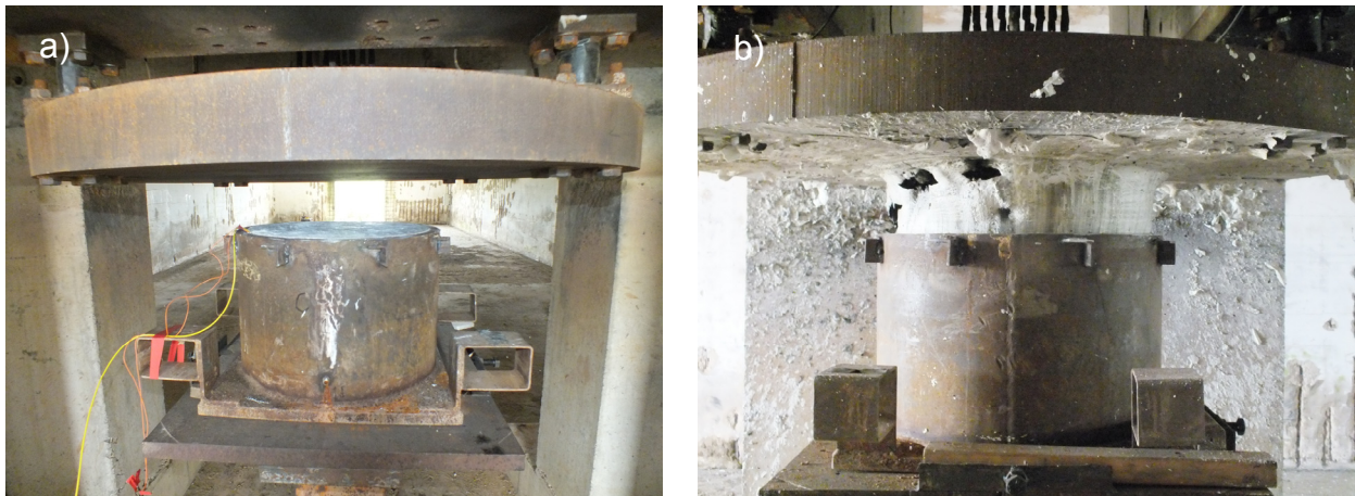
Figure 3: a) pre-test arrangement showing level surface of clay bed, b) post-test showing solidified flow of material across the target plate.
