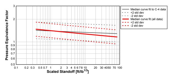
Figure 14: Comparison of original (C-4) and combined (C-4 + PE4) curve fits for pressure.
