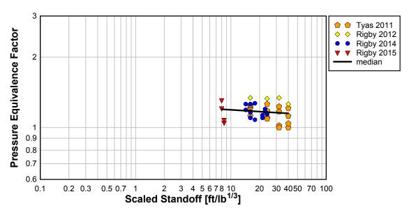
Figure 9: Pressure equivalence data for PE4 vs. scaled standoff.
