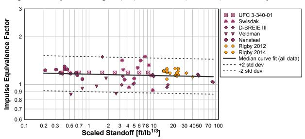
Figure 15: Curve fit to combined C-4 and PE4 data for impulse equivalence.
