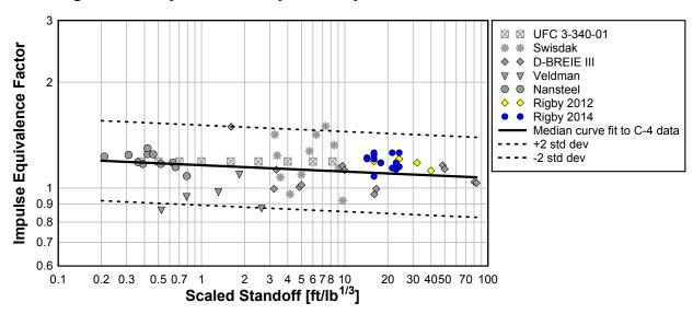
Figure 12: Comparison of PE4 impulse equivalence data to C-4 data and curve fit.
