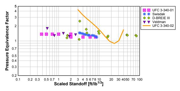
Figure 5: Pressure equivalence from UFC 3-340-02 compared to other sources.
