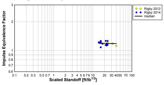
Figure 10: Impulse equivalence data for PE4 vs. scaled standoff.
