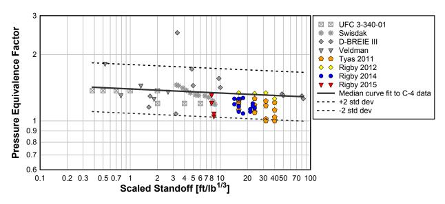
Figure 11: Comparison of PE4 pressure equivalence data to C-4 data and curve fit.
