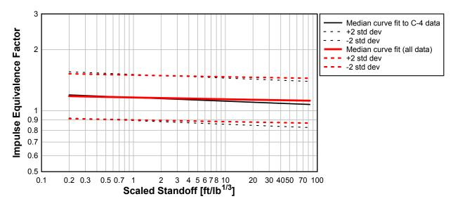
Figure 16: Comparison of original (C-4) and combined (C-4 + PE4) curve fits for impulse.
