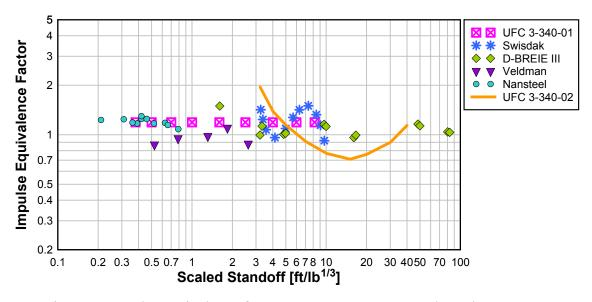
Figure 6: Impulse equivalence from UFC 3-340-02 compared to other sources.
