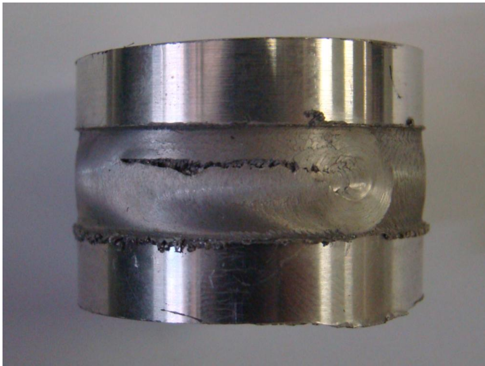
Figure 8 Illustration of the type of weld defect that can occur when the tool pin is misaligned with the centre of the joint and/or tube ovality or eccentricity problems exist, even when the process parameters are appropriate.
