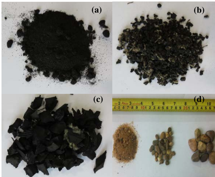
Figure 2: (a) Fine rubber (0-5mm), (b) coarse rubber (5-10mm), (c) coarse rubber (10-20mm) and (d) mineral aggregates used in the experimental programmes.
