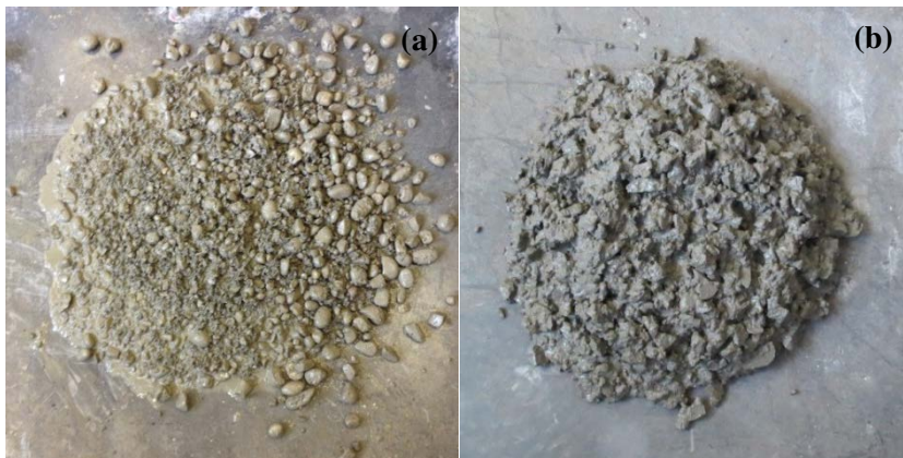
Figure 6: View of flow table test of (a) mix O at 100% FR and (b) mix D at 100% CR.
