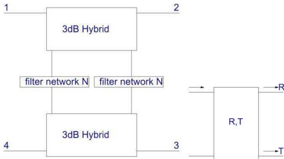
Fig. 1. A single section of a DF and a simplified diagram.
