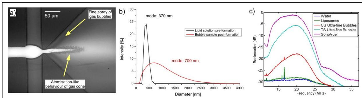
Figure 2: a) Atomisation-like behavior of the gas cone during microspray production. b) Sizing data for supernatant of separated bubble samples. c) US backscatter from samples using a 15 MHz transducer.
