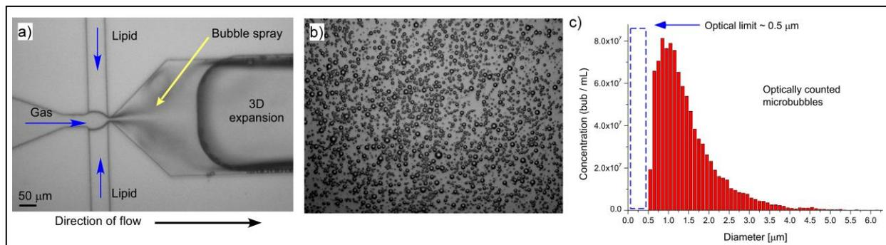
Figure 1: a) Microspray production regime showing 3D expansion in outlet. b) Typical optical image of MBs produced by regime. c) Size histogram of MBs showing the size cut-off in optical counting.
