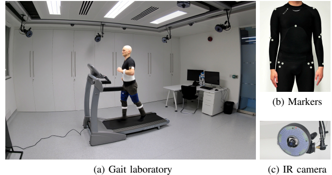
Fig. 1. (a) Gait laboratory equipped with an optical marker-based motion capture system and multi-view camera system for whole body kinematic analysis at The Hamlyn Centre, Imperial College London. The motion of (b) passive retro-reflective markers placed on the upper body are tracked using the optical system's (c) infrared cameras [29].
