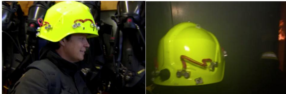
Fig 1. 1st generation Tactile Helmet design undergoing field testing. In right-hand picture the fire-fighter is in a confined smoke-filled space in the South Yorkshire Fire and Rescue training facility.
