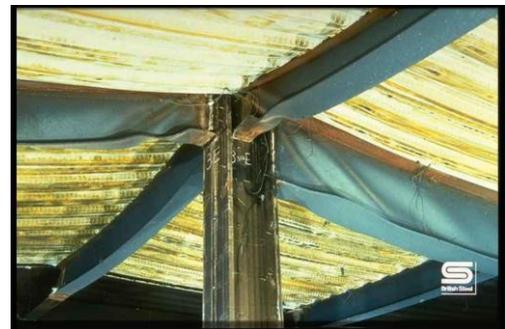
Fig. 1. Shear buckling and bottom-flange buckling in Cardington fire test [4]
