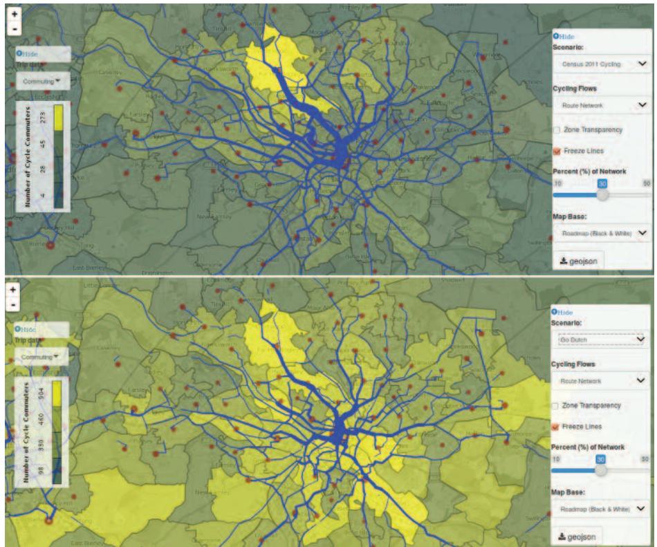
Figure 2: Comparison of cycling flows between the 2011 baseline scenario (above) and the Go Dutch scenario (below)
