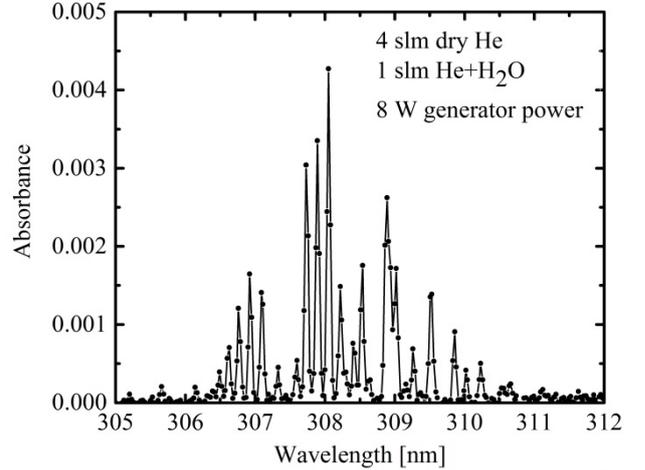
Fig. 3. Typical spectrum of the  $OH\ X^2\Pi(v''=0) \rightarrow A^2\Sigma^+(v'=0)$  transition. Dots indicate measured points. The total He flow is 5 slm of which 1 slm goes through the bubbler. The generator power is 8 W and the corresponding  $OH$  density  $n_{OH} = 2.64 \cdot 10^{20} \text{ m}^{-3}$ .
