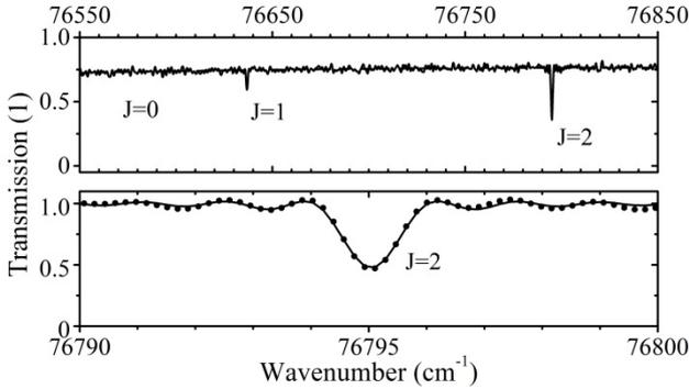
Fig. 2. Typical transmission spectrum of the  $O(2p^4\ ^3P_J \rightarrow 3s\ ^3S^*_1)$  transition for  $J = 0-2$  (top) and  $J = 2$  (bottom). The latter was used for the determination of absolute  $O(^3P)$  densities as described in [7]. The plasma was operated with a generator power of 9 W and 5 slm total He flow, whereas 400 sccm went through the bubbler. The corresponding  $O(^3P)$  density is  $4.0 \cdot 10^{19} \text{ m}^{-3}$ .
