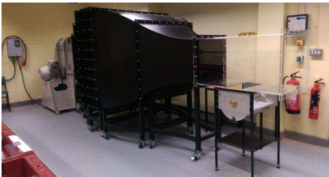
Fig. 1: The constructed open-jet wind tunnel
