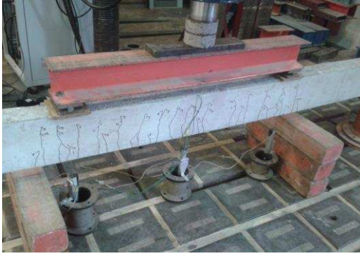
Figure 5 – crack propagation of (a) B-SCC-R and (b) B-SCC-P50
