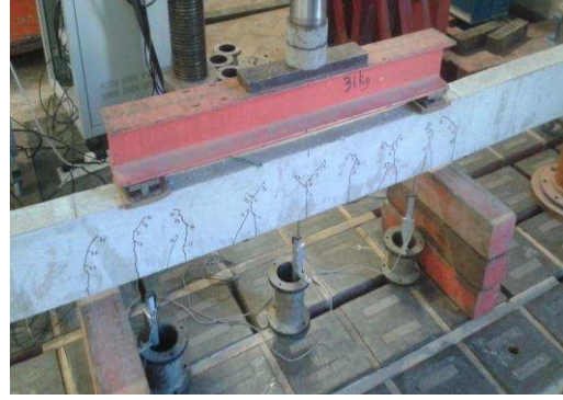
Figure 5 – crack propagation of (a) B-SCC-R and (b) B-SCC-P50
