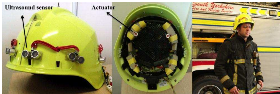
Fig. 1. Our first generation ‘Tactile Helmet’ [3] was composed of a ring of ultrasound sensors and four actuators inside the helmet and was designed to help firefighter’s navigate inside smoked-filled buildings (see Bertram et al. [3] for further details).
