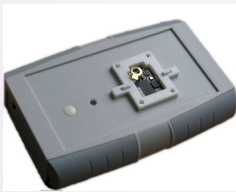
Figure 2. Current solution of reading in the EEG data, a docking station.
