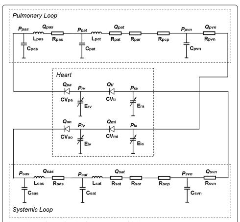
**Figure 4 A sample complete circulatory system model**. (sas: systemic aortic root; sat: systemic artery; sar: systemic arteriole; scp: systemic capillary; svn: systemic vein; pas: pulmonary artery root; pat: pulmonary artery; par: pulmonary arteriole; pcp: pulmonary capillary; pvn: pulmonary vein; lv: left ventricle; la: left atrium; rv: right ventricle; ra: right atrium; mi: mitral valve; ao: aortic valve; ti; tricuspid valve; pa: pulmonary valve).
