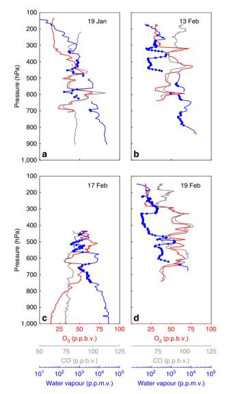
Figure 2 | Ozone, water vapour and CO profiles in the TWP. Sample profiles of 10 s averaged O<sub>3</sub> (red), CO (grey) and H<sub>2</sub>O (blue) from four flights during CONTRAST (**a**,**b**,**d**) and CAST (**c**). Blue circles indicate measurements of H<sub>2</sub>O mixing ratios for which RH <20%. RH is with respect to water and with respect to ice for temperatures above and below 273 K, respectively. Vertical profiles have a characteristic horizontal length of ~300 km.
