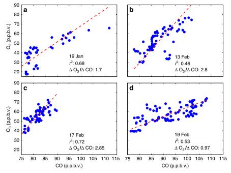
Figure 5 | Enhancement ratios of CO and ozone from CAST and CONTRAST. Regression of CO against O<sub>3</sub> for the data shown in Fig. 2 for pressures between 300 and 700 hPa (**a-d**). The  $\Delta O_3/\Delta CO$  ratio for all profiles suggests significantly aged air, consistent with the back trajectory and photochemical aging analyses. The dashed red line is the best fit via orthogonal linear regression. Flight dates, slope and  $r^2$  values are shown for all panels.
