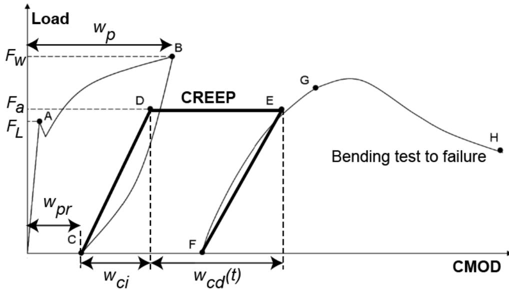
**Fig. 3** Idealized curve obtained in a complete testing process.
