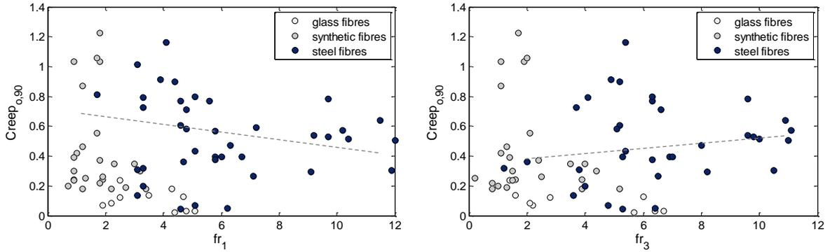
**Fig. 7** Significance of variables  $f_{R1}$  and  $f_{R3}$  vs. creep coefficient  $\phi_0(90)$ .
