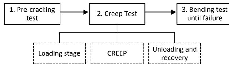
**Fig. 1** General testing procedure.
