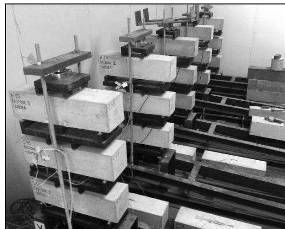
**Fig. 2** Creep test setup.
