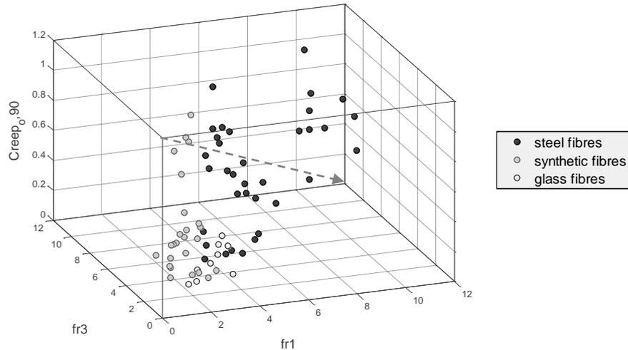
**Fig. 8** 3D plot of variables  $f_{R1}$  and  $f_{R3}$  with creep coefficient  $\phi_0(90)$ .
