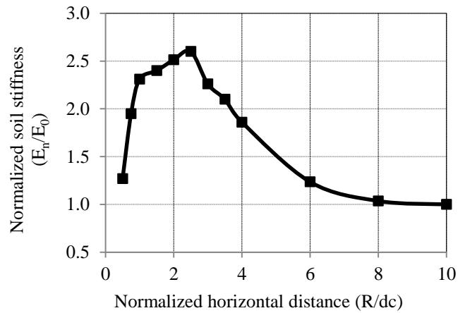
Fig. 9 Variation of stiffness of clay with distance from the column axis (displacement degree = 0.2 m).
