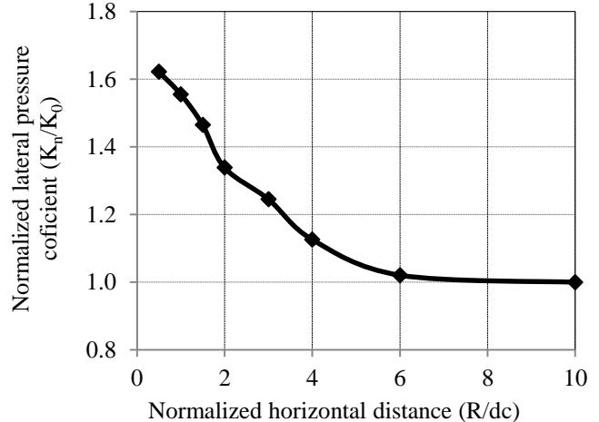
Fig. 8 Variation of stress within the clay with distance from the column axis (displacement degree = 0.2 m).
