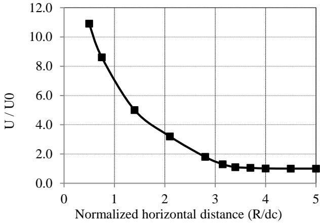
Fig. 7 Variation of excess pore pressure within the clay with distance from the column axis (displacement degree = 0.2 m).
