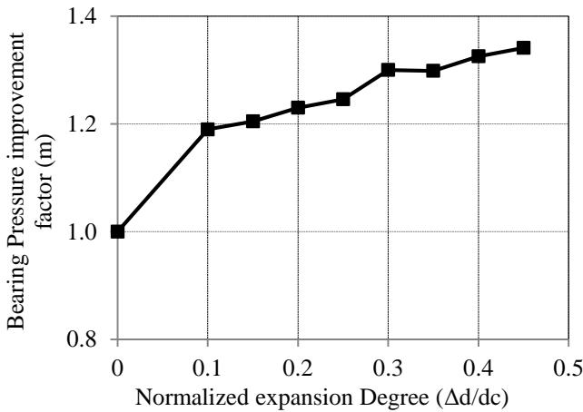
Fig. 10 Effect of expansion degree of the installed stone column on bearing capacity of reinforced footing.
