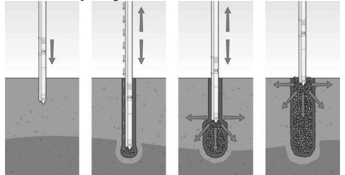
Fig. 1 Vibro displacement by dry bottom-feeding method, [16].
