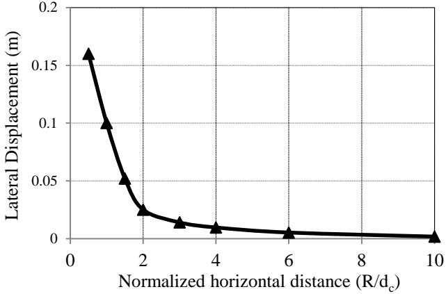
Fig. 6 Variation of lateral displacement within the clay with distance from the column axis (displacement degree = 0.2 m).
