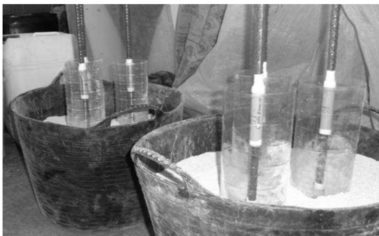
Figure 3. Bottle moulds and rebars prepared and right before casting.
