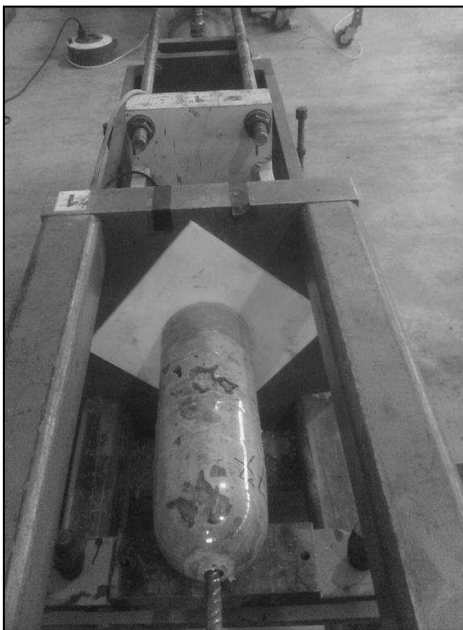
Figure 4. APULOT test carried out on one bottle specimen.
