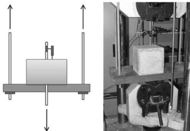
Figure 2: Scheme and picture of the pull out test.
