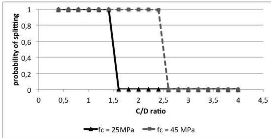
Figure 4: Probability of splitting vs C/D ratio calculated for two compressive strengths.
