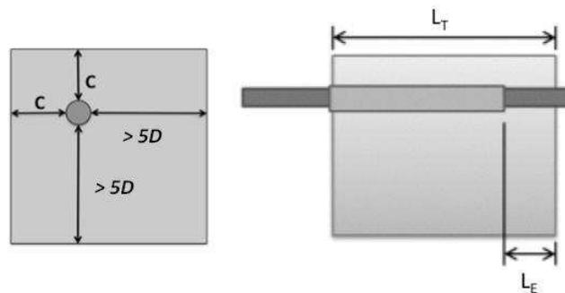
Figure 1: Cross-section (left) and longitudinal section (right) of specimens for pull out test.
