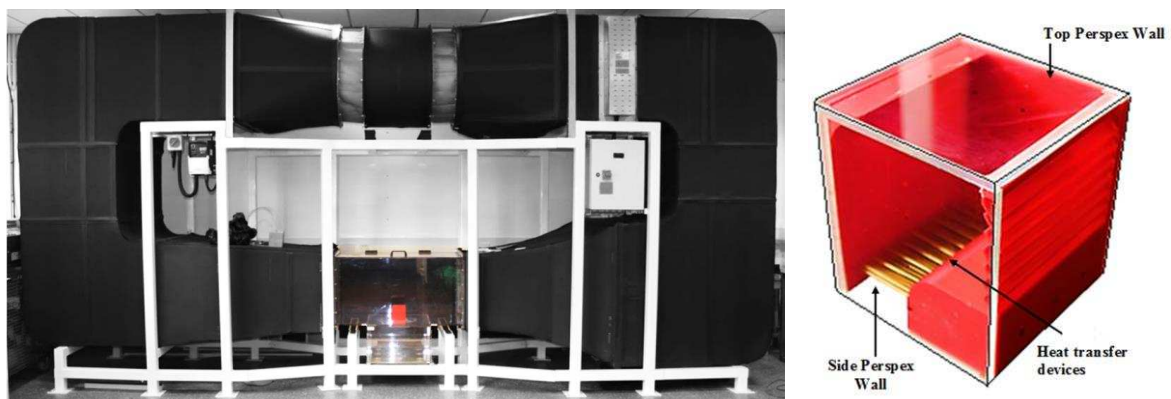
Figure 5: Low-speed wind tunnel (left) 3D printed model (right) [24, 25].
