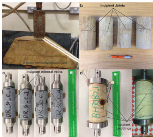
Figure 2. a Sandstone specimens drilled perpendicular to a horizontal incipient joint within a sandstone block, b prepared sandstone specimens with incipient joints, c prepared siltstone specimens with incipient mineral veins, d prepared sandstone specimens with incipient beddings.
