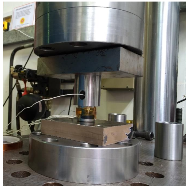
Figure 15 Schematic and photograph of the acoustoelastic constant measurement apparatus. A 10 MHz ultrasonic transducer was used to generate longitudinal wave which propagated through the roller.
