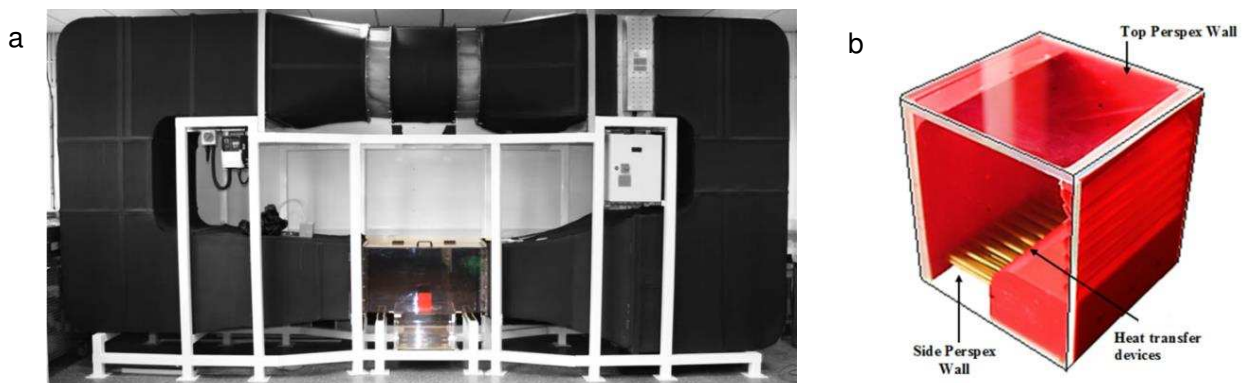
Fig.4 (a) closed-loop wind tunnel (b) 3D printed wind catcher model.
