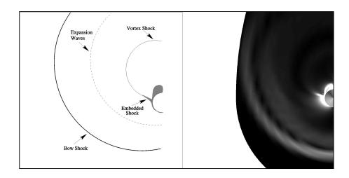
Figure 3: Computed density gradient ( $\nabla \rho$ ) on crossflow plane at x/D=5.5, and interpretation
