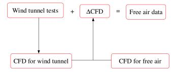
Figure 13: A diagram for CFD correction of wind tunnel data
