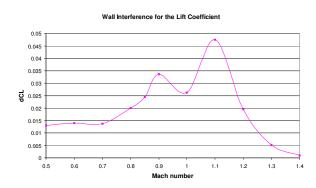
Figure 15: Lift coefficient difference between free air case and wind tunnel solid wall case
