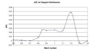
Figure 16: Lift coefficient difference between solid wall case and solid wall + support case
