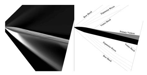
Figure 2: Computed symmetry plane density gradient ( $\nabla \rho$ ), surface skin friction lines and interpretation.
