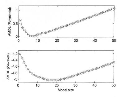
Figure 7. AMDL index versus the number of model terms for polynomial model (the plot at the top) and wavelet model (the plot at the bottom) identification described in Example 2. The AMDL criterion for the wavelet model was calculated in the normalised space.
