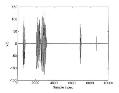
Figure 10. The difference  $\mathcal{E}(t) = y(t; b_2 + \delta) - y(t; b_2)$  produced by the noise-free model (27a), described in Example 3, where  $\delta = 10^{-4}$ .
