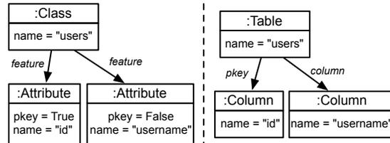
Fig. 1. Two consistent CD and RDB models
