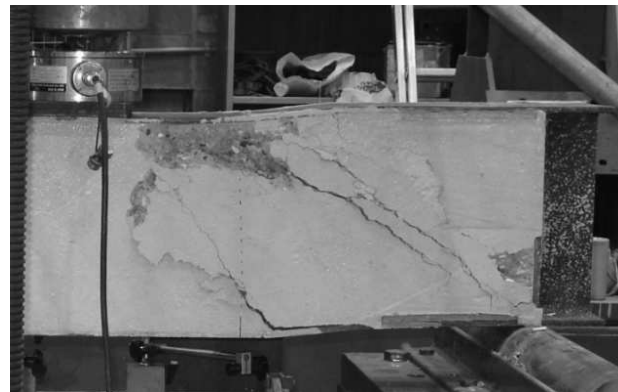
Figure 8. USFB No.2 at Failure point.
