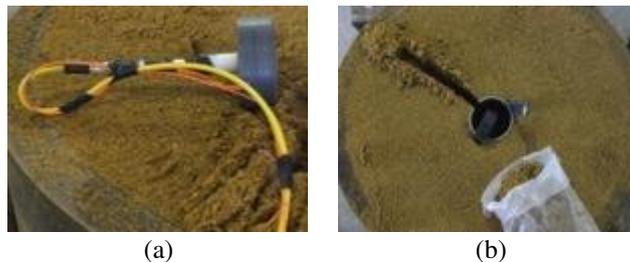
**Figure 5.** Images taken from charge preparation process: (a) non-el detonator and break-wire umbilical prepared for burial (b) charge hole and umbilical trench prepared
