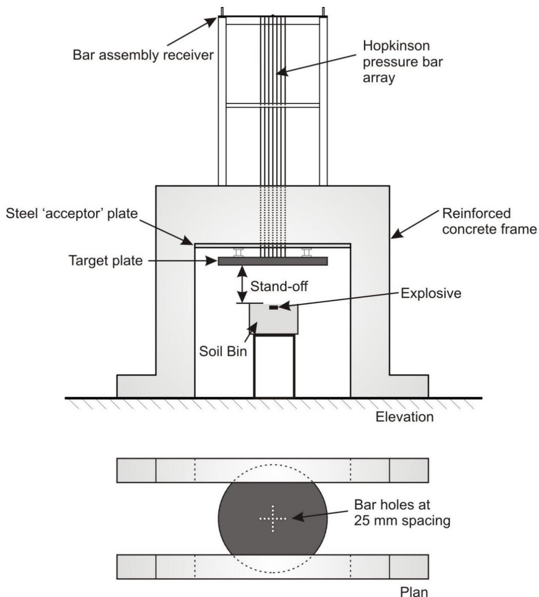
**Figure 2:** Test frame schematic – not to scale
