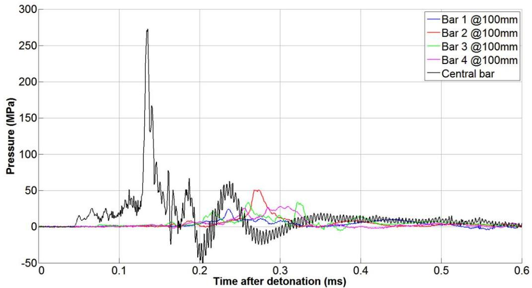
**Figure 4.** Test A, pressure-time history, top detonation
