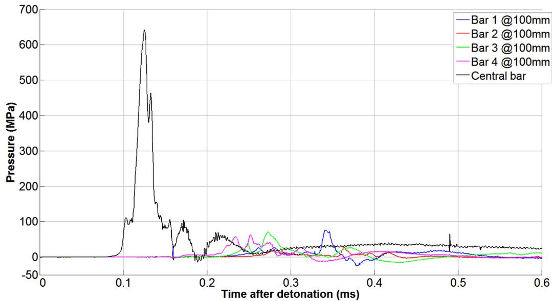
**Figure 6.** Test B, pressure-time history, base detonation
