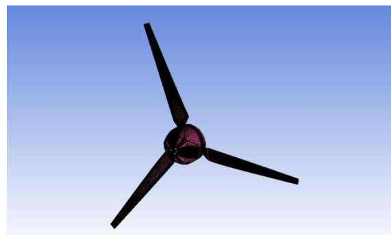
Figure 1 Mesh of the turbine in the CFD simulation
