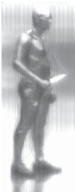
Fig. 3 A passive outdoor image of an individual holding a metal knife concealed in a newspaper obtained at 94 GHz. Although there is little spectral information available over this frequency range, differences in the electromagnetic properties of skin, explosives, metal, etc., can allow the detection of weapons or concealed packages 13 . (Courtesy of Roger Appleby, QinetiQ, UK.)
