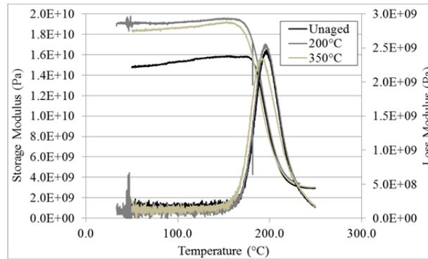
**Figure 3.** Storage and loss moduli results obtained in DMA tests (3-point bending configuration) for three considered conditions.
