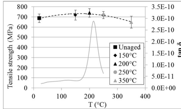
**Figure 1.** Tensile strength of CFRP samples subjected to different ageing conditions. The value represented for each condition is the average of 5 measurements.
