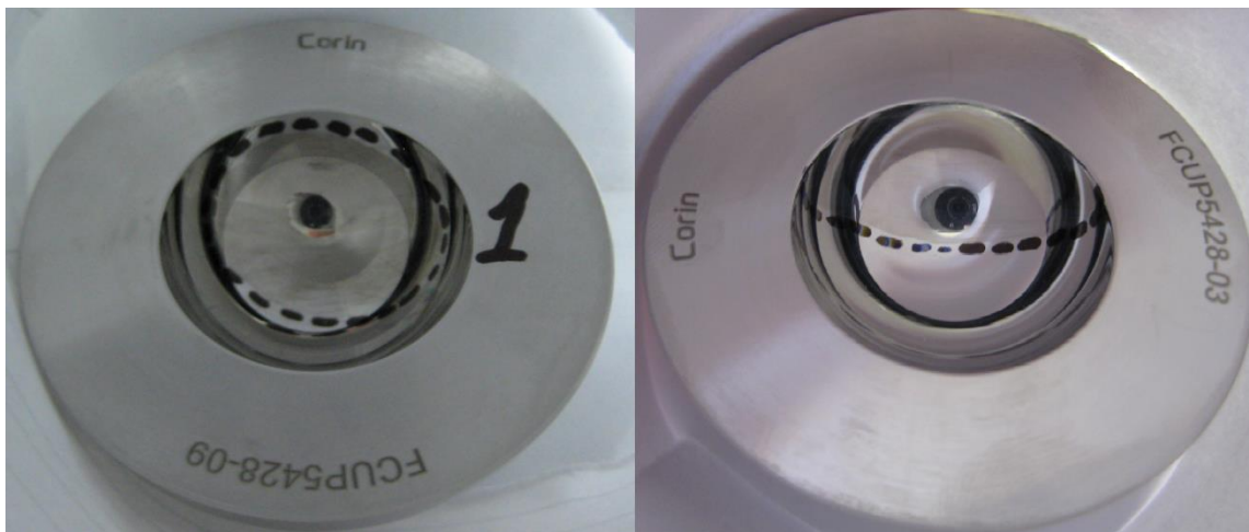
Figure 9: Photographs of the 28mm inner diameter acetabular cups showing the wear area (within dotted line) under standard conditions with 45° inclination angle (left) and the wear area under steep inclination angle (right). Under steep inclination angle the wear area intersected with the rim of the acetabular cup.
