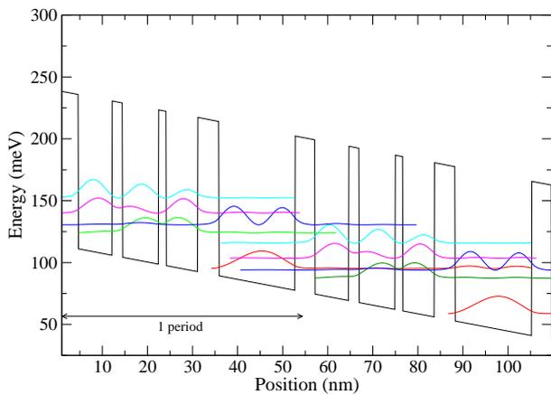
Fig. 3. Energy-band diagram of the ambipolar THz QCL in Ref. 5 at 7 kV/cm without the tight-binding approach. This leads to an extended state 1 wavefunction providing an unrealistic resonant LO phonon current path.
