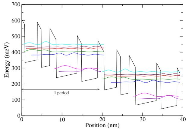
Fig. 5. Energy-band diagram of the GaN THz QCL in Ref. 8 at a forward bias of 80 kV/cm with the tight-binding scheme to obtain the localized wavefunctions shown.
